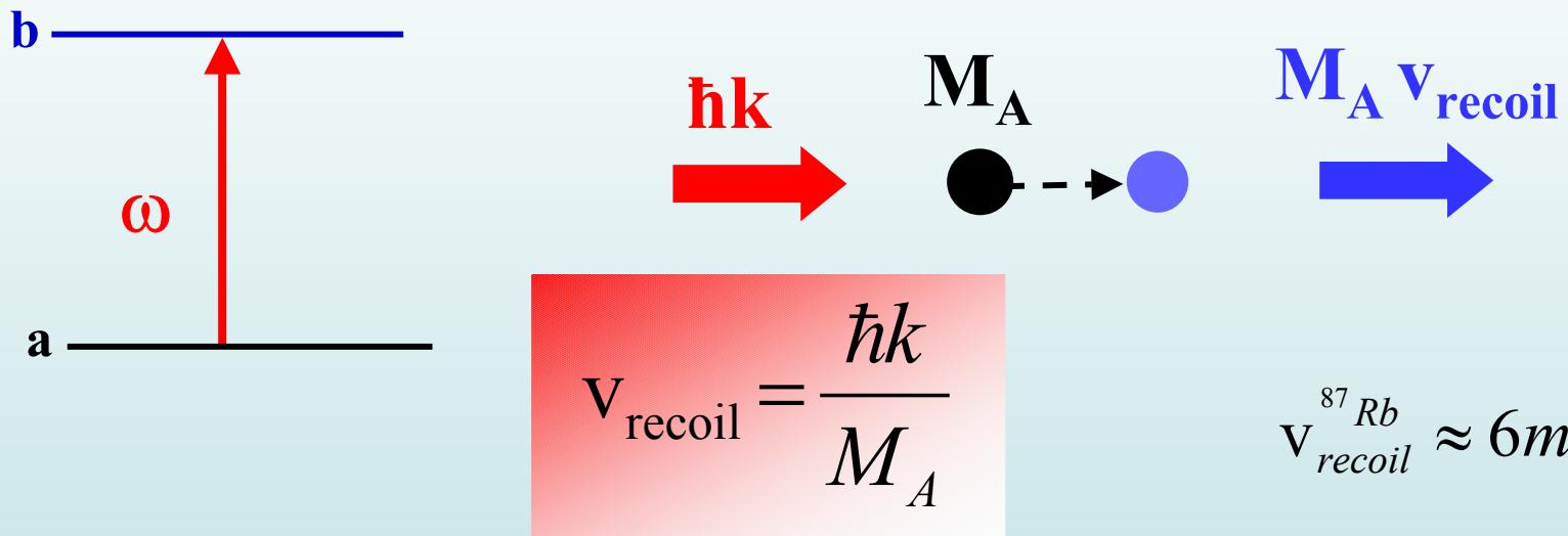
measurement of  $v_{\text{recoil}}$  and  $k \Rightarrow h/M_A$
