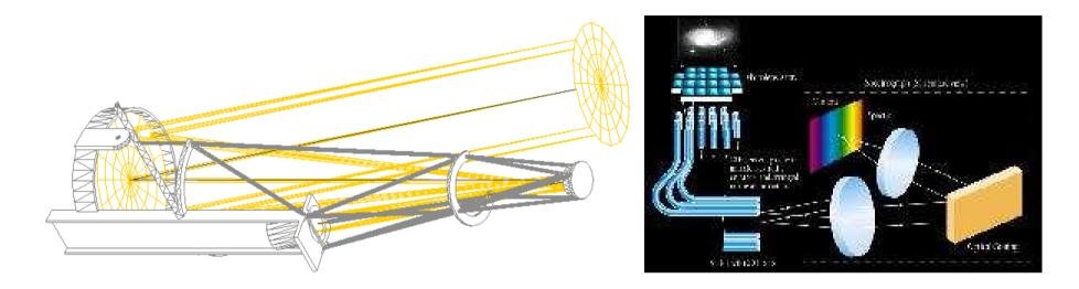
A two meters class telescope will allow a 1 Gauss sensitivity with a 1 arcsec resolution in 5 mn integration time. Better spatial resolution will be possible for high coronal magnetic fields in the very low corona above active regions.
