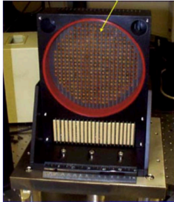
349 actuators on 7 mm spacing
