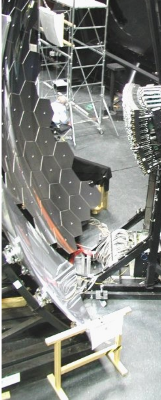
Schmidt Telescope using 11 m 2 mirrors
