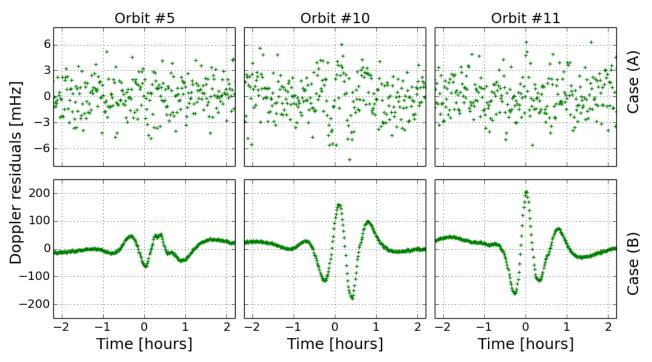
In case (B) signatures appears: the static gravity field cannot absorb the signal coming from the acoustic modes, which emerge from the noise.
