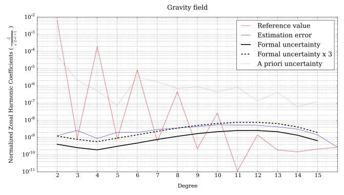
Neglecting the modes lead to an error slightly higher than 3-sigma.
