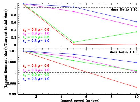
FIGURE 2: Amount of accretion as a function of impact speed for the four cases of bulk density and coefficient of restitution and two separate mass ratios. On the plot values greater than 1.0 represent accretion while values less than 1.0 represent erosion.
