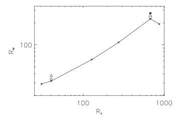
Fig. 1.—Critical magnetic Reynolds  $R_M^c$  for dynamo action (solid line) inferred from direct numerical simulations (crosses), as a function of  $R_V$  (Ponty et al. 2005). The position of the runs discussed in Table 1 are indicated by symbols: run A (diamond), A' (triangle), B (square), and B' (asterisk).
